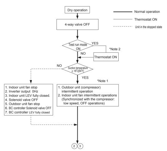
\*Note 1.When the indoor unit inlet temperature exceeds 18°C [64°F], the outdoor unit (compressor) and the indoor unit fan start the intermittent operation simultaneously. When the indoor unit inlet temperature becomes 18°C [64°F],or less, the fan always runs (at low speed). The outdoor unit, the indoor unit, and the solenoid valve operate in the same way as they do in the cooling operation when the compressor is turned on.
