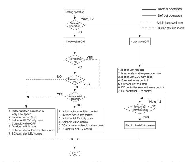
\*Note 1. When the outdoor unit goes into the defrost mode, defrost command is sent to the BC controller and indoor units. Upon reception of the command, the indoor units will go into the defrost mode. When defrosting is completed and upon receiving the signal that indicates the completion of defrosting, indoor units will resume the heating operation.
