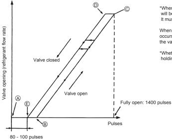
\*When the power is turned on, the valve closing signal of 2200 pulses will be output from the indoor board to LEV to fix the valve position. It must be fixed at point  ${\widehat{\triangle}}$
