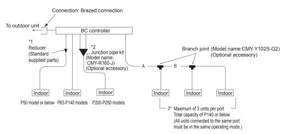
The ports of the BC controller accommodates the pipes on P63-P140 models of indoor units. To connect other types of indoor units, follow the procedure below.
