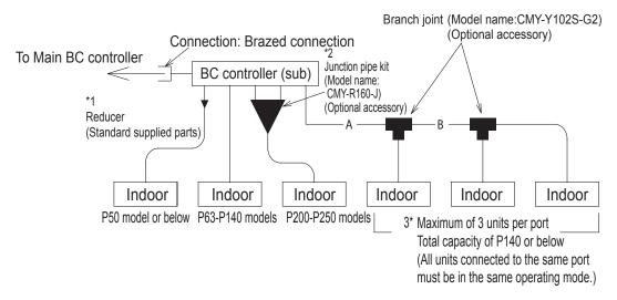
The ports of the BC controller accommodates the pipes on P63-P140 models of indoor units. To connect other types of indoor units, follow the procedure below.
