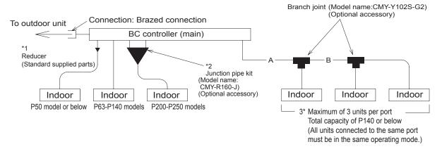
The ports of the BC controller accommodates the pipes on P63-P140 models of indoor units. To connect other types of indoor units, follow the procedure below.
