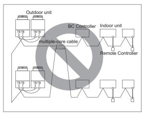
TB3: Terminal block for indoor-outdoor transmission line TB7: Terminal block for centralized control
