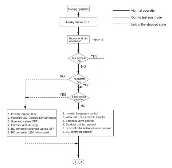
\*Note 1. The indoor fan operates at the set notch under cooling mode regardless of the ON/OFF state of the thermostat.
