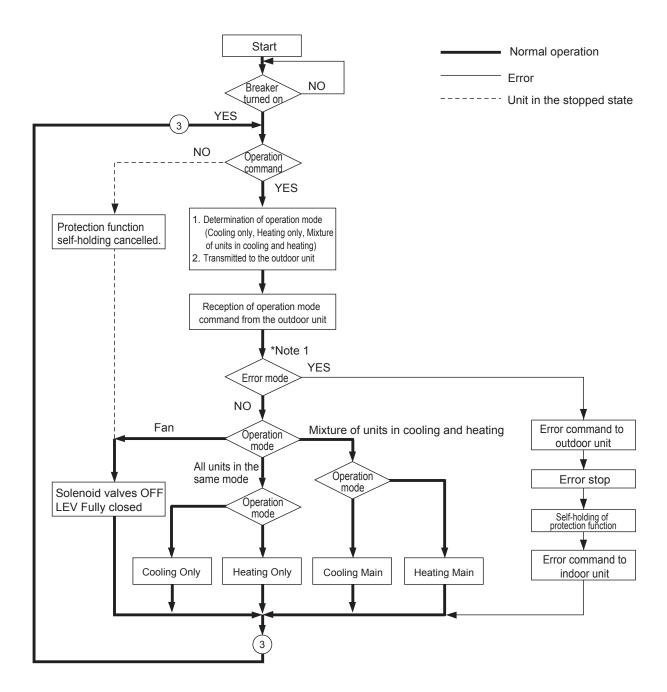
Note 1. The system may go into the error mode on either the indoor unit side or the BC controller or outdoor unit side. If some of the indoor units are experiencing a problem, only those indoor units that are experiencing the problem will stop. If the BC controller or the outdoor unit is experiencing a problem, all the connected units will stop.
