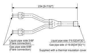
Note) Use the flare nut that is supplied with the BC controller.
